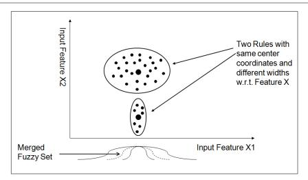
Fig. 7 Embedded fuzzy sets (for input feature X) due to projection concept and as one cluster lie over the other with respect to dimension Y; the merged set indicated by dotted line, yielding an inexact representation of the local data clouds w.r.t. dimension X
