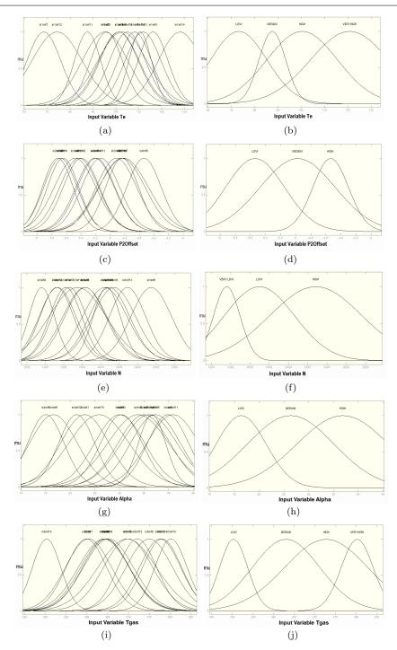
Fig. 11 Left side: final fuzzy partitions obtained for (from top to bottom) Te, P2offset, N, Alpha and Tgas when using full precise EFS; right side: the final partitions obtained for the same variables when detecting fuzzy set redundancies and eliminating these in connection with EFS
