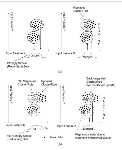
Fig. 9 (a): Cluster misplacement of upper cluster due to alignment along dimension X, as the merged set is back-integrated; (b): updating upper cluster with new data makes situation worse: also the lower cluster is misplaced according to dragging effect and alignment and the update of the upper cluster is not sufficient as starting from misplaced position
