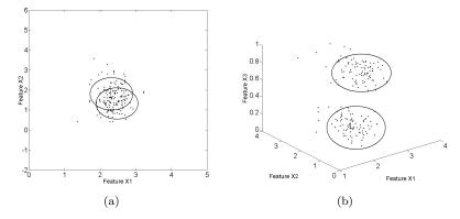
Fig. 3 (a): two over-lapping clusters in the projected two-dimensional feature space (b): clusters significantly torn apart in the three dimensional feature space, as no overlap along the third dimension (Feature X3) is present
