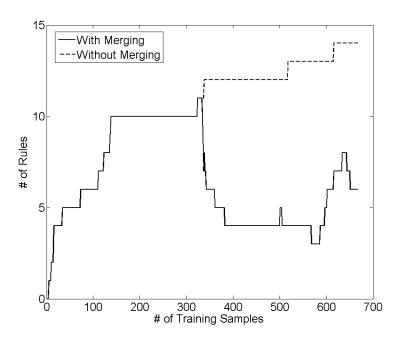
Fig. 10 (Evolution progress on the number of rules for NOx data set when using conventional EFS (without redundancy deletion) as shown in dotted line versus evolution progress on the number of rules when using EFS with coupled rule merging in case of strongly overlapping rules (solid line)
