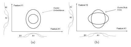
Fig. 4 (a): one cluster is fully embedded in another cluster  $\rightarrow$  overlap degree is equal to 1 as the intersection of the fuzzy sets is at membership degree 1 in both dimensions (b): cluster cross, reverse embedded along both dimensions  $\rightarrow$  overlap degree is equal to 1
