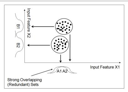
$\textbf{Fig. 6} \ \ \text{Strongly overlapping fuzzy sets in the X dimension because of projection onto the axes}$
