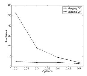
Fig. 12 The effect of different settings of the vigilance parameter on the number of extracted rules in case when rule merging is switched off (line with crosses) and on (line with circles)
