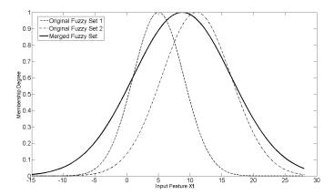
Fig. 8 Merging of two Gaussian fuzzy sets (dashed and dotted dashed lines) to a new fuzzy set according to (21)
