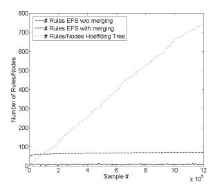
Fig. 15 Development of the number of rules over time for EFS without merging (dashed line), with merging (solid line) and Hoeffding trees (dotted line) — note the linear increase of the latter and the logarithmic saturation of EFS without merging at around 70 rules; EFS with merging achieves 7 rules in average
