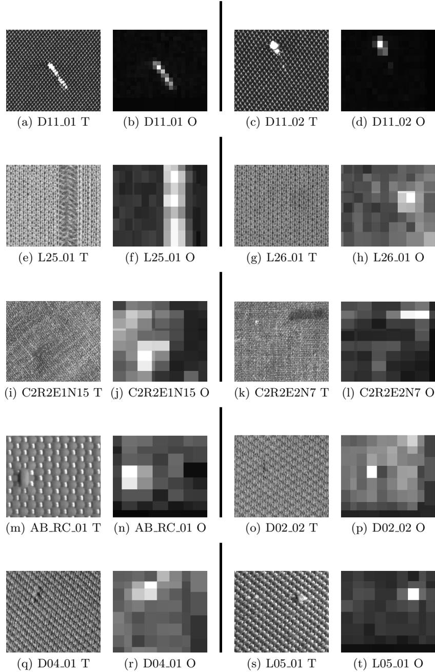
**Fig. 1.** Examples of the applicability test on textile defect images. For each example the test image (T) as well as the output (O) of the algorithm is shown. Reference images are not shown. The algorithm output is for illustration purposes not thresholded.
