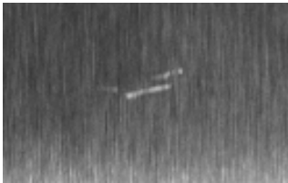
Figure 1. stainless steel plate with noise surface and scratch
