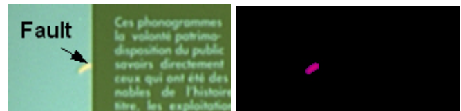
Fig. 1. Left Image: original image with a faulty dot; right image: the deviation image from (the fault-free) master
