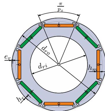
Fig. 3. Cross-section of the rotor for the considered optimization problem.
