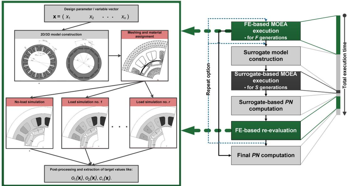
Fig. 5. An overview of the surrogate-based optimization process used in the present research. There are three hypothetical targets that must be considered: two optimization objectives ( $o_1$  and  $o_2$ ) and one constraint ( $c_1$ ).
