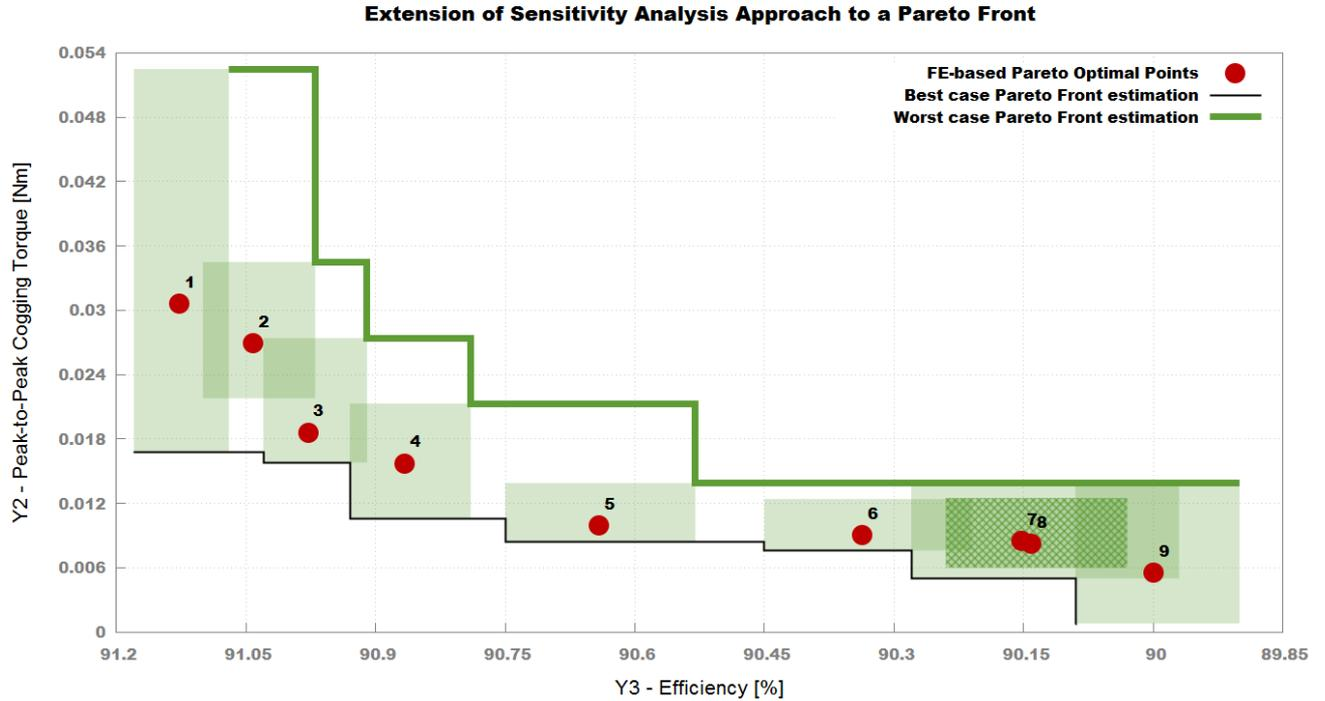
Fig. 8. The extension of our surrogate-based sensitivity analysis approach to an FE-based Pareto front. The transparent min-max sensitivity box associated with point 8 is also hashed in order to better distinguish it from the larger encompassing box associated with point 7.
