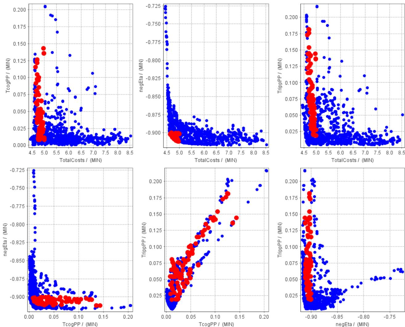
Fig. 7. Two-dimensional objective space projections of the 1004 Pareto non-dominated designs that were discovered after performing the multi-objective optimization phase. The highlighted designs simultaneously have an efficiency higher than 90% and a cost lower than 5 Euros.
