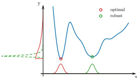
Fig. 1. Robust vs. optimal rated performance: While for rated operation the solution indicated by the red circle performs best, this is not necessarily the case when tolerances occur. An example for a Gaussian distribution of the selected design parameters and their impact on the output is presented.
