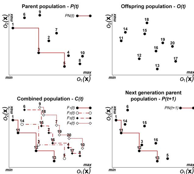
Fig. 4. Conventional optimization strategy - for instance, the multi-objective minimization problem is solved by applying NSGA-II, a very well-known multi-objective evolutionary algorithm that relies on a strategy intended to generation-wise move its population towards the Pareto-optimal set.
