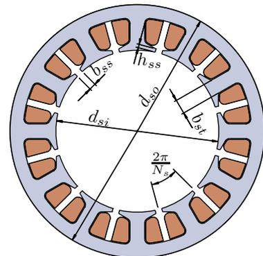
Fig. 2. Cross-section of the stator for the considered optimization problem.
