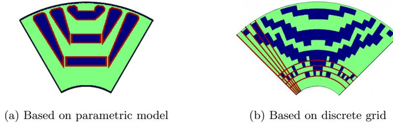
Fig. 1: Example of two cross-sections of rotor designs. Light green parts denote iron elements and dark blue parts denote air gaps.
