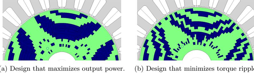
Fig. 5: Rotor designs obtained by DECMO (with a real-value encoding) for the realistic DTO scenario.
